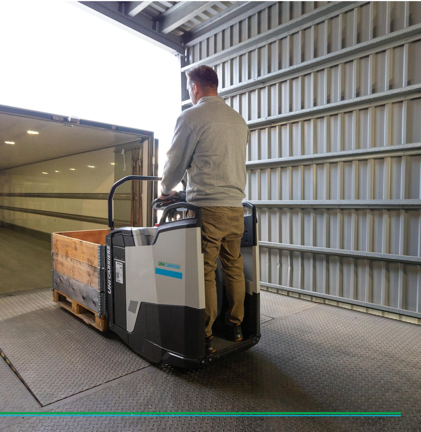
Tiller arm design permits comfortable operating position with optimum hand protection.
